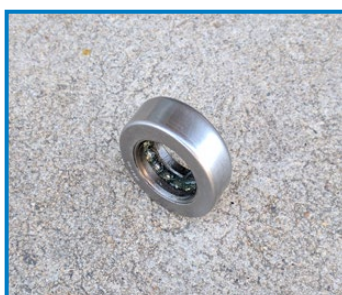
MAIN DRIVE SHAFT THRUST BEARING Item #303
